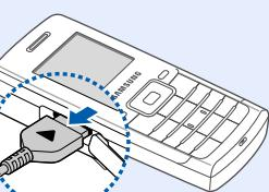
**Note:** Do not remove the battery from the phone without unplugging the travel adapter first. Otherwise, the phone may be damaged.
