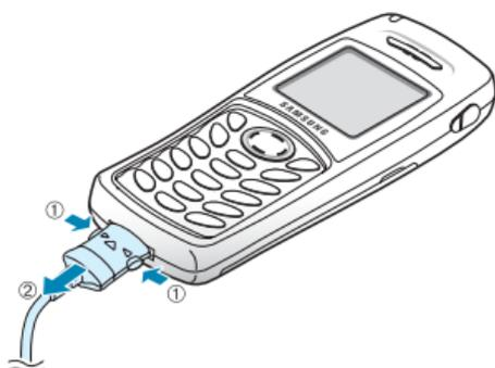
**Note:** Do not remove the battery from the phone while it is charging without first unplugging the adapter. If you do so, the phone may be damaged.
