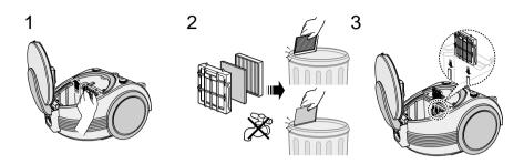
**NOTE**: Do not allow the filter to become clogged as this may cause power reduction or may damage the motor.
