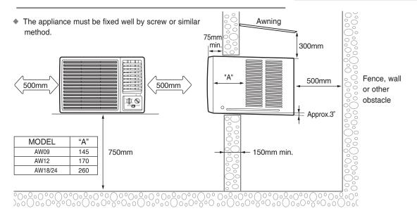
If the wall is greater than 150mm thick, cut the wall back on a 45° angle if possible.
