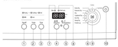
During DRYcycle, displayed remaining time may be increased or decreased. Such a condition is not a system failure, but a DRYfunction optimization process.
