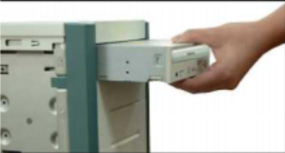
1. Make sure that the PC is powered off and disconnected from any power source.
