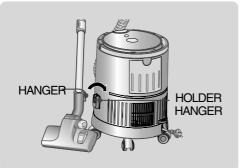
For easy storage, this vacuum cleaner has a hanger system built on the body, which will keep the Tube, Suction Hose and Floor Nozzle in a vertical position.
