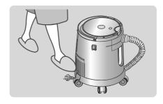
**REWINDING**After disconnecting the plug from the electrical outlet, press the cord rewind button lightly with your toe. The cord will automatically rewind.
