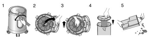
Turn the Suction Hose Clamper counterclockwise and pull it out.
