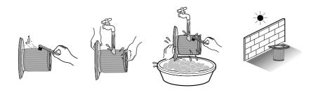
After using, if the filter is full of dust, clean it as picture and use it again.
