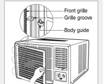
The air conditioner has two or three grille grooves depending on the model.
