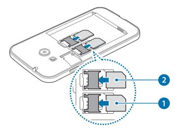
► Single SIM models: Insert the SIM or USIM card with the gold-coloured contacts facing downwards.
