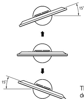
The angle of the PDP can be up to 15 degrees left/right.
