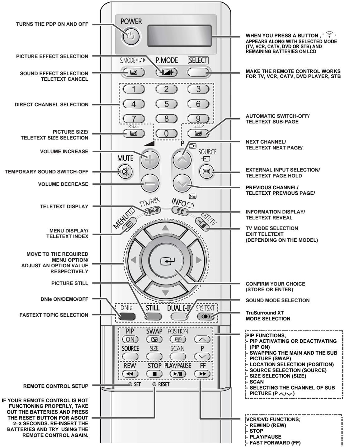
IF YOUR REMOTE CONTROL IS NOT FUNCTIONING PROPERLY, TAKE OUT THE BATTERIES AND PRESS THE RESET BUTTON FOR ABOUT 2-3 SECONDS. RE-INSERT THE BATTERIES AND TRY USING THE REMOTE CONTROL AGAIN.
