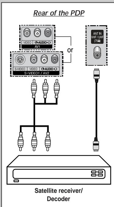
In order to watch television programmes broadcast via a satellite network, you must connect a satellite receiver to the rear of the PDP. Also, in order to descramble a coded transmission signal, you must connect a decoder to the rear of the PDP.
