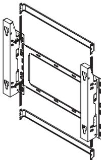
The wall mount bracket is delivered separately. Please tighten the captive screw in the direction of the arrow after assembling the bracket.
