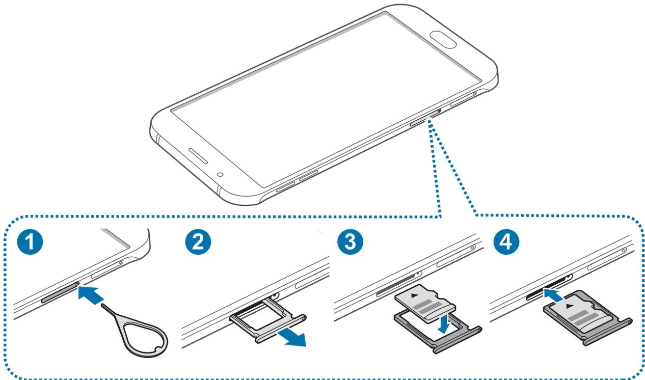
1 Insert the ejection pin into the hole on the memory card tray to loosen the tray.
