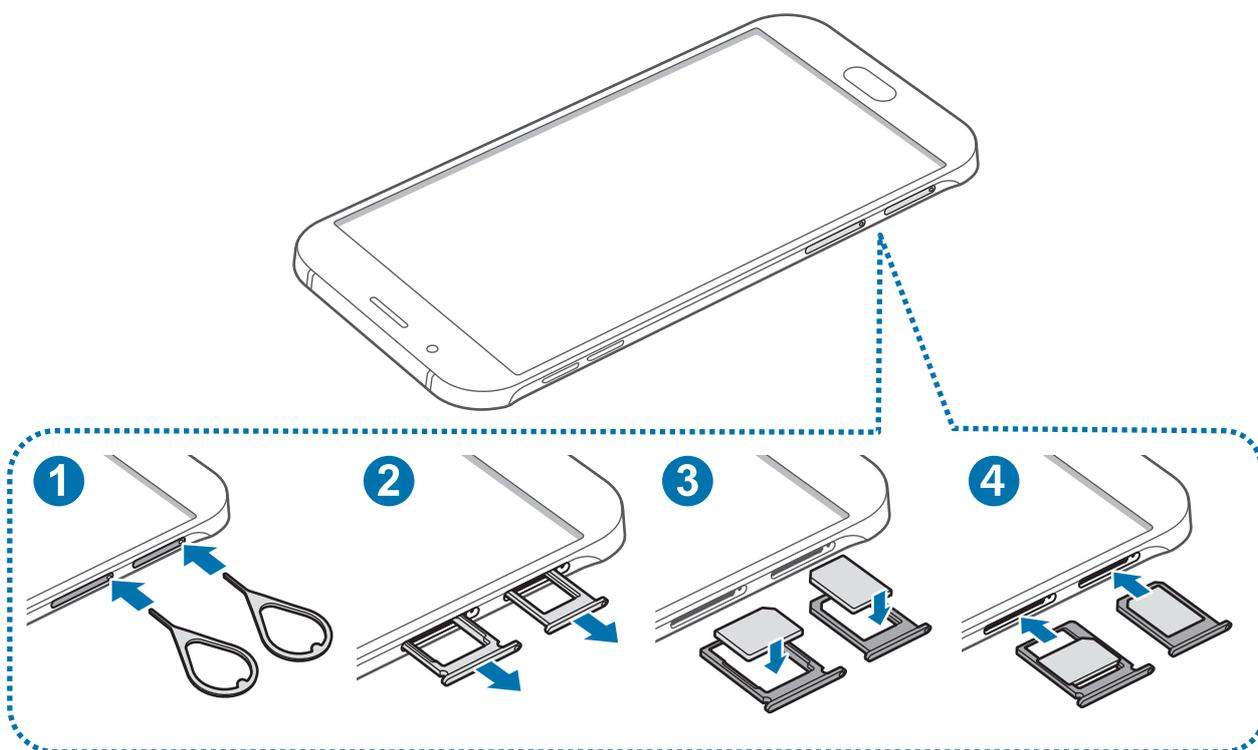
**1** Insert the ejection pin into the hole on the SIM card tray to loosen the tray.
