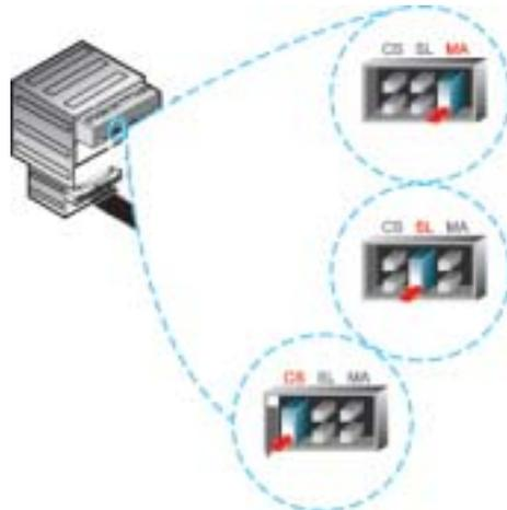
Connect a jumper to the rear side of the CD-R/W.
