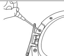
8. Move the position of the screw at the back of the door-hinge.
