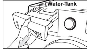
2. Remove the condensed water inside the water-tank.
