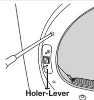
12. Now, move to the right side of the product and fasten the two screws holding the front-frame and the two screws holding the lever-holder.
