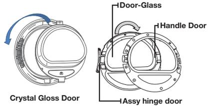
6. Fasten the 16 screws in the correct positions. Fasten the 6 screws and replace the air seal. (Only for Crystal Gloss door models)
