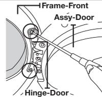
4. Remove the 16 screws. Disassemble the air seal and remove the 6 screws (3 flat head screws at the top and 3 round head screws at the bottom). (Only for Crystal Gloss door models)
