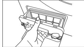
4. If the heat exchange filter is not cleaned regularly, a display indicator will be turned on or blinked as a reminder. If so, check the heat exchanger filter and clean it to make sure that the filter is not blocked with lints.
