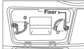
3. Remove the Heat Exchanger Filter.
