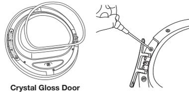
5. After removing the screw, rotate the Assy hinge door, the handle door by 180° as shown in the figure.
