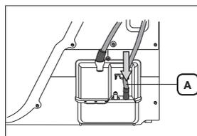
3. Connect accessory hose(long drain hose) (B) to the hole next to the hole that is connected to drain hose (A).
