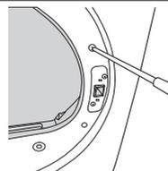
13. Align the door with the fixing holes.
