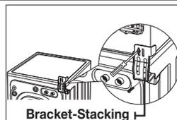
5. Install dryer and bracket on washer
