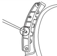
10. Remove the two screws holding the front-frame at the left.
