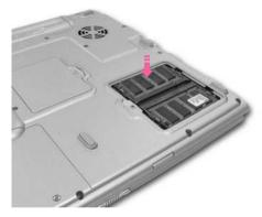
5. Close and fix the memory-module compartment cover using a screwdriver.
