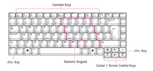
**Special Function Keys:** The <Fn> key activates special functions when pressed in combination with other keys.
