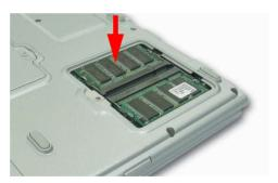
3. Close and fix the memory module compartment cover using a screwdriver.
