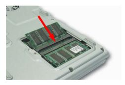
2. Push the memory module in until the module clicks into place. If the memory module is not fixed completely, gently push the memory down while pressing the memory module tabs outward.
