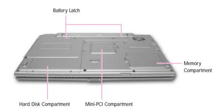
Mote The removal of the HDD is not allowed. To replace the HDD, please contact your service center. Wireless LAN/Bluetooth module(optional) is installed in the mini PCI compartment. After doing so, when you turn the system on, the system examination program is executed automatically.
