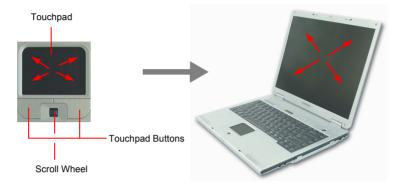
The touchpad on your computer allows you to move the pointer on the LCD screen, just like a mouse that is used with a desktop computer. The touchpad buttons allow you to take actions with the pointer, such as selecting an item or executing a command. The scroll wheel between the touchpad buttons moves the displayed area up and down within a window.
