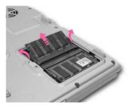
3. Align the new memory module connectors accordingly and slide it into the slot at a 30° angle.
