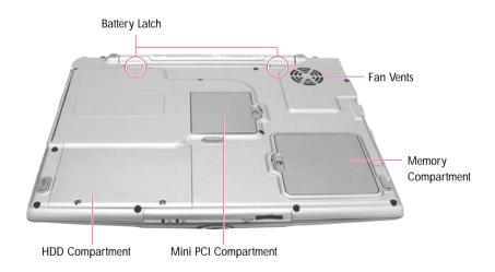
Caution The removal of the HDD is not allowed. To replace the HDD, please contact your service center. The Mini PCI compartment is used for the installation of the optional wirevice center. The M less LAN module.
