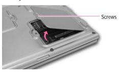
2. Push the memory module tabs outward to pop the memory module outward. Pull the module out at an angle of about 30°.
