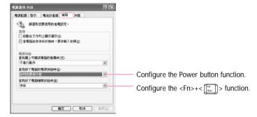
Caution : When the Power button is configured to put the system into Power-Saving Mode, manually shutting down the computer requires the Power button to be pressed and held for more than 4 seconds.
