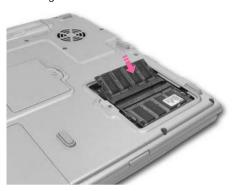
4. Push the memory module in until the module clicks into place. If the memory module is not fixed completely, push the module while pressing the memory module tabs outward.
