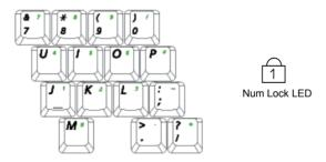
Press <Fn>+<F11> to turn on the embedded numeric keypad. The numeric functions of the keypad are enabled and the Num Lock LED turns on. (See "Reading the Status Indicators" on page 22 for the location of the Num Lock LED.)
