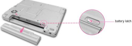
Caution: In X10 plus model, slide left battery latch outward( 1), then remove the battery while holding the right battery latch outward(
