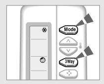
The Sleep Timer can be used when you are cooling/heating your room to switch the air conditioner off automatically after a period of six hours.
