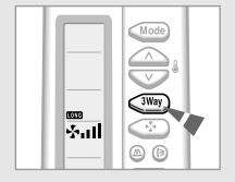
You can use the Long cooling/heating function when you wish to make the cool/warm air run to every corner in your room, especially when you are away from the air conditioner.
