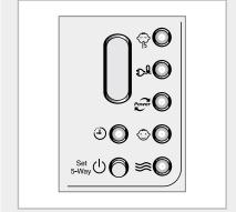
2 To stop the operating, press the ( ) (On/Off) button until all indicators turn off.
