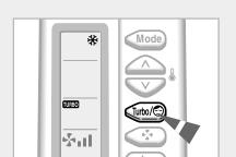
The Turbo cooling function is used to cool your room as quickly as possible.
