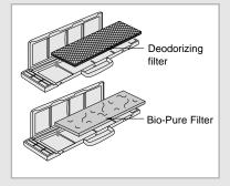
The air conditioner can be fitted with a deodorizing and Bio-Pure filter to remove minute dust particles or odours. The service life of the filter is approximately three months depending on the time during which the air conditioner is used.
