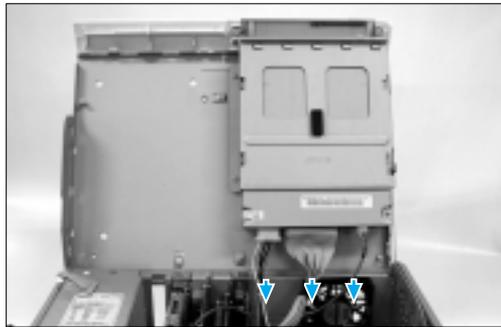
3. Remove the CD Drive bracket by unscrewing the 4 screws that holds the bracket in place.
