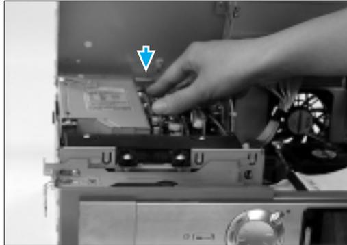
**Warning** : **If it is difficult to insert the card because the connectors are too long** You can insert the card more easily if you rest the cover on the Cover Stopper(Lid safety Latch).
