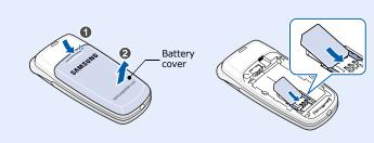
2. Install the battery and reattach the cover.
