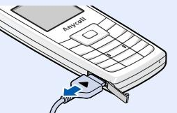
**Note:** Do not remove the battery from the phone without unplugging the adapter first. Otherwise, the phone may be damaged.
