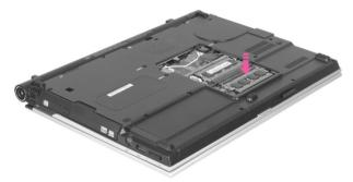
5. Close and fix the memory-module compartment cover using a screwdriver.
