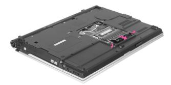
3. Align the new memory module connectors accordingly and slide it into the slot at a 30° angle.
