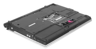
4. Push the memory module in until the module clicks into place. If the memory module is not fixed completely, push the module while pressing the memory module tabs outward.
