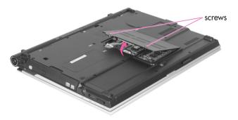
2. Push the memory module tabs outward to pop the memory module outward. Pull the module out at an angle of about 30°.
