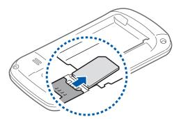
► Insert the SIM card by aligning it (notch to the lower right and gold contacts down) and then sliding it into its slot.
