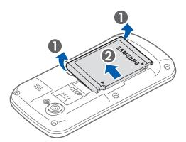
▶ Insert the battery by aligning the gold contacts on the phone and the battery and then gently pressing the battery into place.
