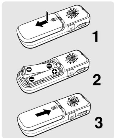
**1** Slide the battery cover in the direction of the arrow as shown in the diagram and open it.
