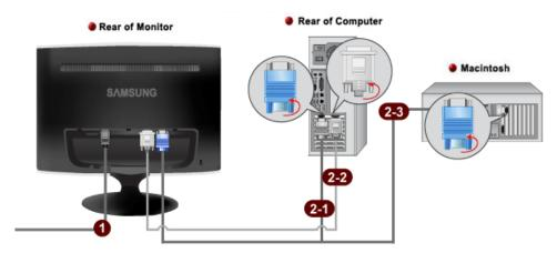
Onnect the power cord for your monitor to the power port on the back of the monitor.
