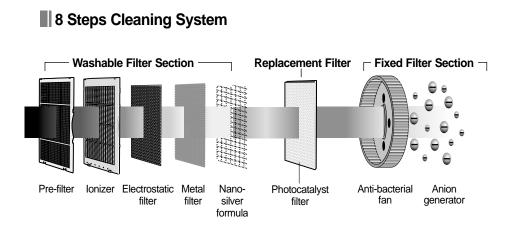
Note The Metal filter is coated with the Nano-silver particles.
