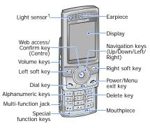
1. Controls the backlight brightness to save the battery power.
