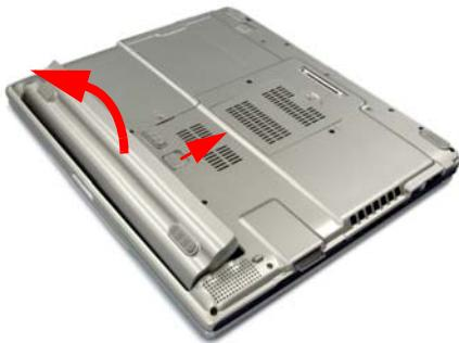
4. To attach the battery, place the battery into the system. Check that the battery latch is in the Lock position().
