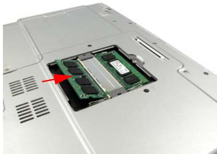
2. Push the memory module in until the module clicks into place. If the memory module is not fixed completely, gently push the memory down while pressing the memory module tabs outward.
