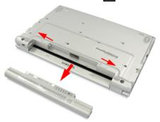
**4.** To install the battery again, insert the battery into the battery compartment of the system and slide the right battery latch in the direction of closed( ) to fix the battery.
