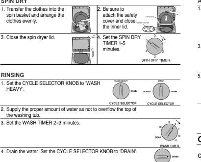
5. Repeat this cycle until drain water is clean. (2~3 cycles)
