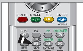
Press the "STILL" button to freeze a moving picture into a still one. Press again to cancel.
