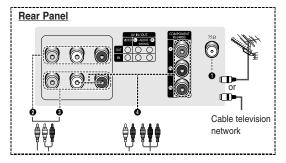
Whenever you connect an audio or video system to your television, ensure that all elements are switched off. Please be sure to match the color coded input terminals and cable jacks.
