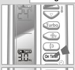
The On Timer enables you to switch on the air conditioner automatically after a given period of time. You can set the period of time from 0.5 hour to 24 hours.
