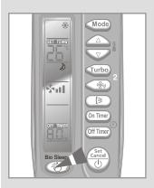
Bio Sleep mode helps users to fall asleep well after going to bed whether being too hot to sleep or being awakened by coldness. The Bio Sleep Mode can be selected only when the air conditioner is switched on or off in cool mode.
