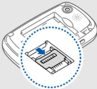
3. Lift the memory card cover and insert a memory card with the label side facing up.
