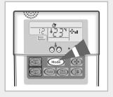
3 To adjust the temperature, press the Temperature buttons one or more times until the required temperature is displayed. Possible temperatures are between 18°C and 30°C inclusive.
