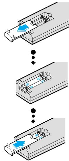
**1** Remove the battery cover on the back of the remote by pressing down and sliding the cover in the direction of the arrow.
