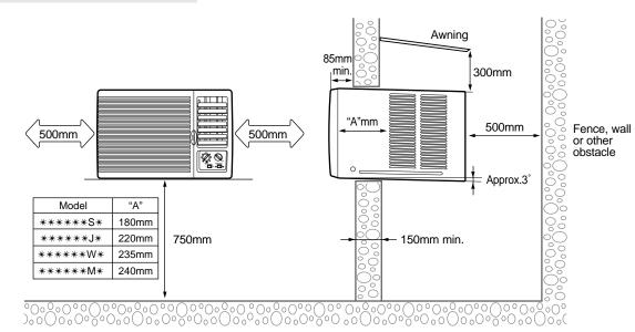
If the wall is greater than 150mm thick, cut the wall back on a 45° angle if possible.
