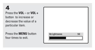
■ After adjusting an item, the gauge will automatically disappear (after about 5 seconds).
