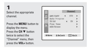
Press the CH ▼ button three times to select "Fine tune", then press the VOL+ button.
