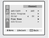
Press the VOL+ and VOLbuttons to adjust the fine tuning.
