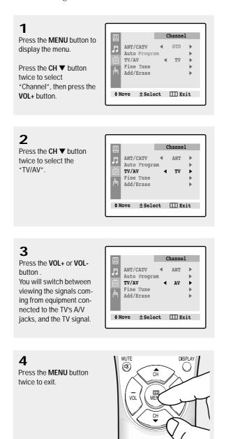
Note: In the AV mode, the software available in all of the NTSC, PAL & SECAM devices is displayed on the screen after automatically judging the TV system (For model CT-21K3W).
