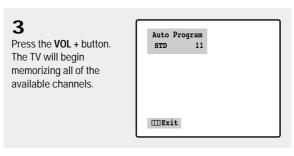
■ The TV automatically cycles through all of the available channels and stores them in memory. This takes about one to two minutes. Press the MENU button at any time to interrupt the memorization process and return to the Channel menu.
