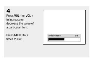
■ After adjusting an item, the gauge will automatically disappear (after about 5 seconds).
