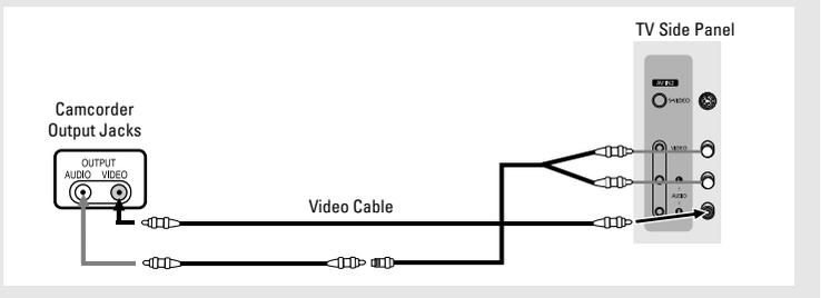
The audio-video cables shown here are usually included with a Camcorder. (If not, check your local electronics store.) If your camcorder is stereo, you need to connect a set of two cables.
