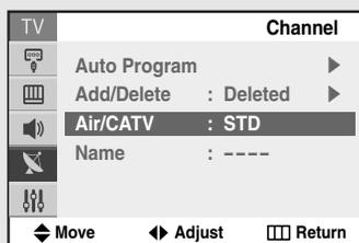
$\blacktriangleleft$  STD, HRC and IRC identify various types of cable TV systems. Contact your local cable company to identify the type of cable system that exists in your particular area.
