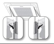
Clean the grille and Air filter with a vacuum cleaner or soft brush. If dust is too heavy, then rinse it with running water and dry it in a ventilated area.
