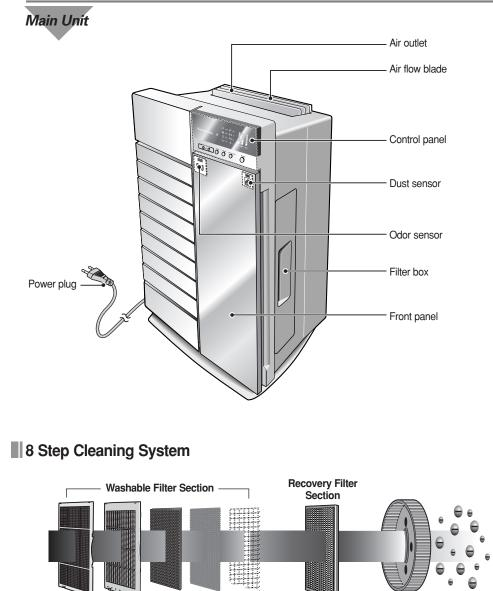
Ionizer Electrostatic Metal Nano TiO<sub>2</sub> Anti-bacterial Anion filter filter silver photocatalyst fan generator formula filter
