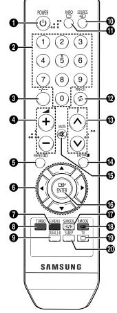
POWER Used to switch the TV on and off.
