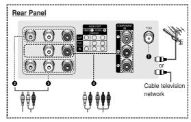
Whenever you connect an audio or video system to your television, ensure that all elements are switched off. Please be sure to match the color coded input terminals and cable jacks.
