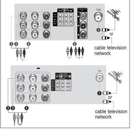
Whenever you connect an audio or video system to your television, ensure that all elements are switched off. Please be sure to match the color coded input terminals and cable jacks.
