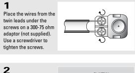
Plug the adaptor into the TV ANTENNA terminal on the bottom of the back panel.
