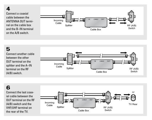
After you've made this connection, set the A/B switch to the "A" position for normal viewing. Set the A/B switch to the "B" position to view scrambled channels. (When you set the A/B switch to "B," you will need to tune your TV to the cable box's output channel, which is usually channel 3 or 4.)
