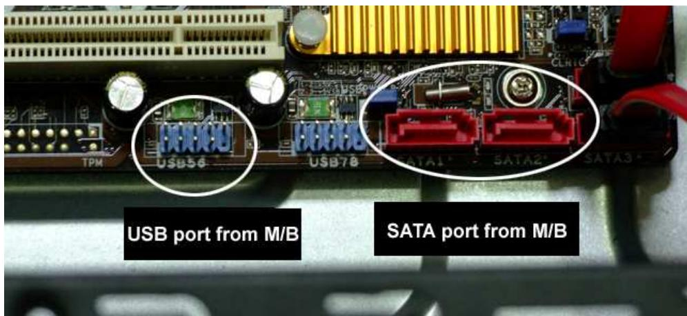
3. Connect the USB and SATA cables to the USB and SATA ports on the motherboard to the back plate adapter. Please note for the USB connection that connector side with the red marked cable corresponds to pin 1. Use the shortest SATA cable available because of the maximum allowed total cable length (1m).
