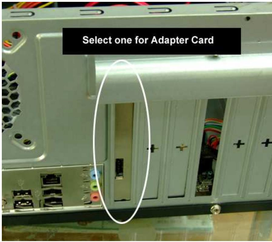
6. Reassemble the PC case and connect a Power Over eSATA cable to the external port on the card.
