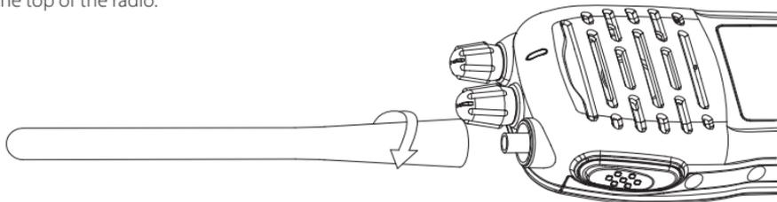
**Note:** Do not operate the radio or press PTT key without an antenna installed.
