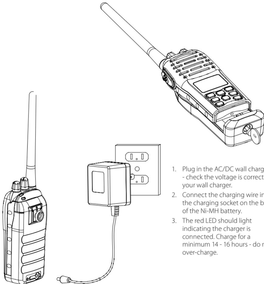
1. Plug in the AC/DC wall charger - check the voltage is correct for your wall charger.
