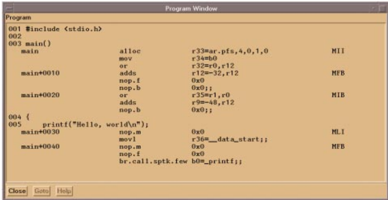
Figure 5-2. xski 's Program Window Showing Intermixed C and IA-64 Assembly Code
