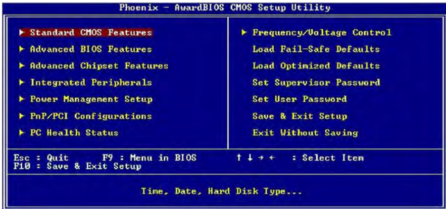
Figure 4-1 CMOS Setup Utility Main Screen
