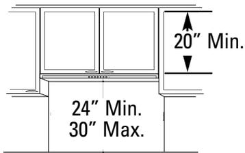
The cabinet must be at least 20" high between the bottom frame and the inside top. A custom cabinet or modifications to a different size cabinet may be required to accommodate the hood housing.
