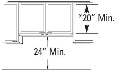
\*The cabinet must measure at least 20" from the bottom frame to the inside top. The hood housing will occupy the interior cabinet space.
